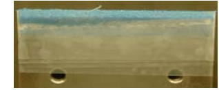
Figure 2: Photo of talc interlayer before deformation
